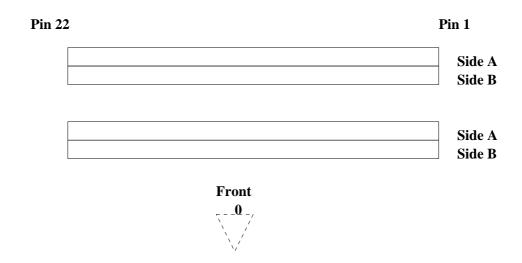
Components are normally mounted onto Side A of the PCB within the cartridge.
