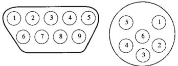
Note: Connections as viewed from back of connector (Solder side)
