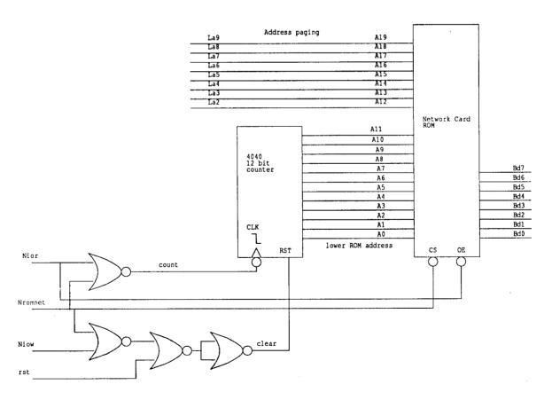
Figure 1. Recommended ROM addressing circuit.
