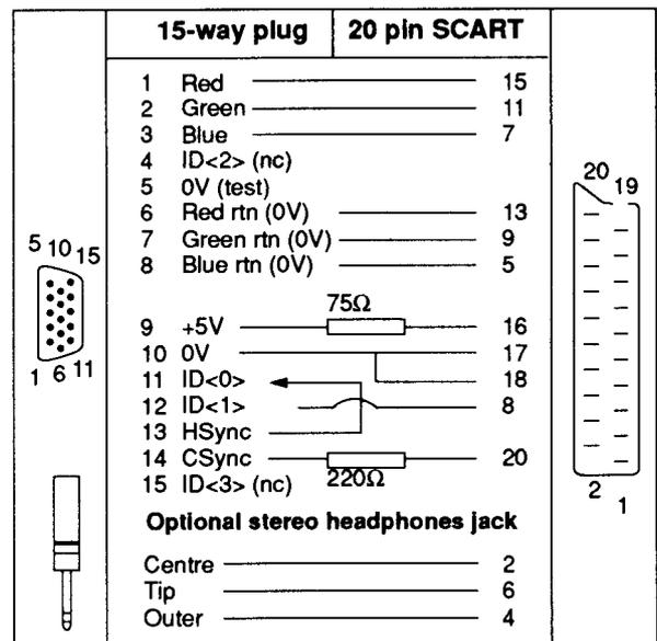
The 220Ohm resistor results in a CSYNC signal of approximately 1V peak on pin 20 of the SCART connector. The 750hm resistor results in a blanking signal of approximately 2.5V dc on pin 16 of the SCART connector.
