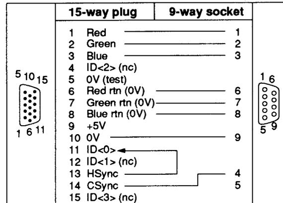
**Note:** The HSYNC to ID[0] connection will make the monitor type 0 modes available and the computer will generate a composite sync signal.
