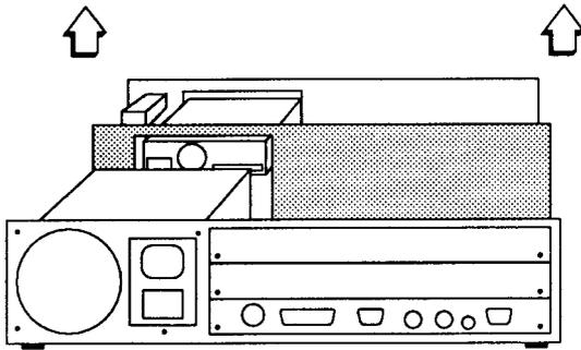
6 Once you have removed the tray, you can remove the floppy disc drive (item 77) and the hard disc drive (item 78) by turning the tray over and unscrewing the four screws which hold each drive in place. Take care to observe all anti-static precautions when storing the disc drives.
