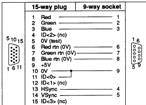
**Note:** The ID[0] to 0V connection will make the monitor type 3 modes available and the computer will generate separate sync signals.
