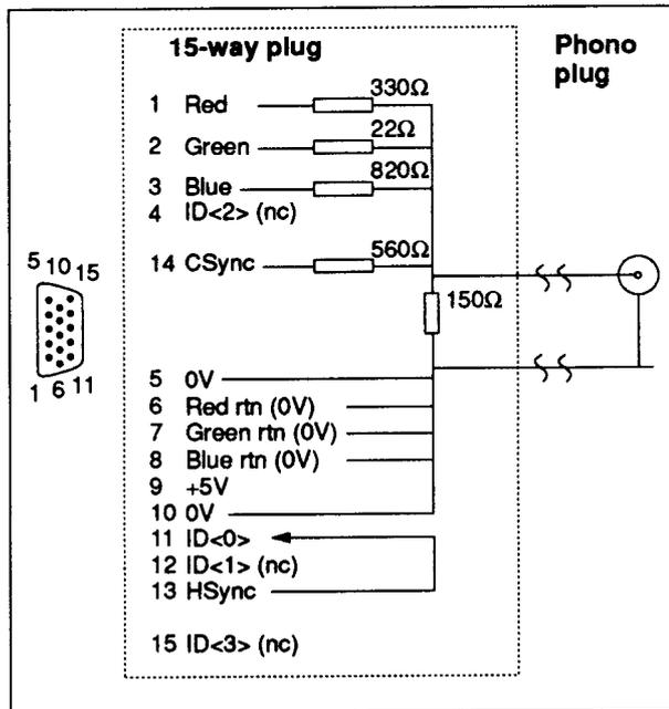
**Note:** The HSYNC to ID[0] connection will make the monitor type 0 modes available and the computer will generate a composite sync signal.
