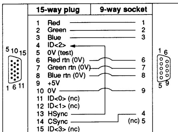
**Note:** The HSYNC to ID[2] connection will make the monitor type 1 modes available and the computer will generate a composite sync signal.
