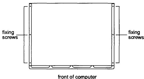
5 Rest the main unit on its base again and slide the lid (item 24) backwards to the rear of the unit. Remove the lid completely.
