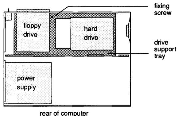
5 The tray has two tabs which fit into the front slots of the unit and four clips, two at each side, holding the tray in place. Remove the tray from the main unit by grasping both ends of the support metalwork. The whole
