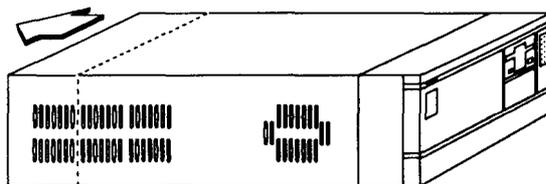
6 Some models of the A5000 have an EMC case shield (item 29) which fits over the case. To remove this shield, unscrew the five fixing screws on the right hand side of the unit, as seen from the rear. The shield has interleaved tabs which fit into the edges of the case. Slide the shield off the main unit carefully; there is a hole on the top to help you slide the shield off by inserting a screwdriver.
