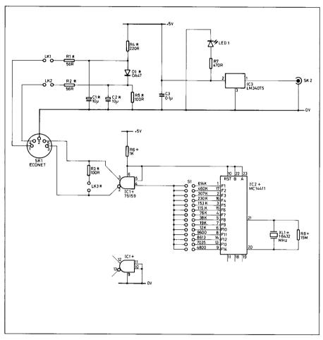
Components marked \* are fitted on terminator boxes only. Components marked + are fitted on clock boxes only.
