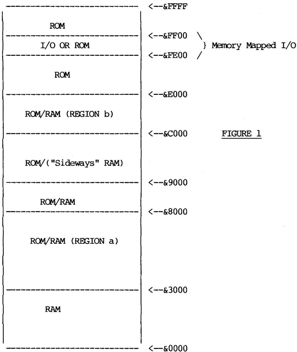
The current memory map is dictated by the contents of the two latches, ROM SElect and ACCess CONtrol located at &FE30 and &FE34 respectively.
