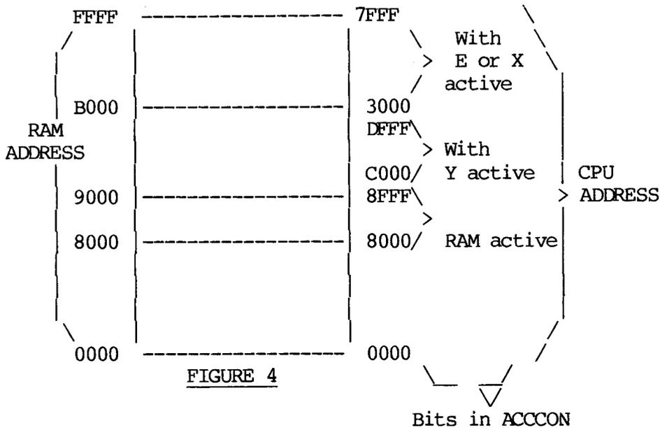
A further 64k byte of RAM is available as 4 pages of 16K byte from &8000 to &BFFF. The ROM slots 4,5,6 and 7 are not active when this RAM is link selected to be active.
