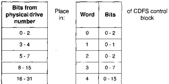
All bits of the control block not mentioned above must be initialised to zero. The whole process can be done as follows:
