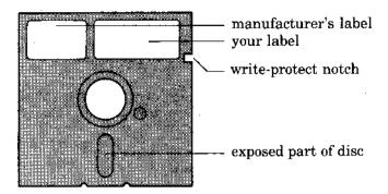
At the side of most discs is a notch, called the write-protect notch. This can be covered with a plastic adhesive patch which protects all the information on it from being wiped off by mistake. While this patch is on, you cannot save anything on the disc. You may wish to protect important discs you use, and you will find spare write-protect patches in your boxes of new discs.
