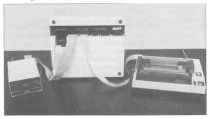
4 Hold the second processor upright immediately to the right of the micro 5 Hold the loose end of its ribbon connector like this, with the small v-shaped marking to the right
