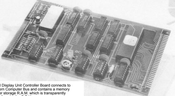
The Acorn Visual Display Unit Controller Board connects to the Standard Acorn Computer Bus and contains a memory mapped character storage R.A.M. which is transparently written to or read from by the C.P.U.
