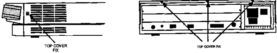
Figure 1: Removing the screws holding the top cover
