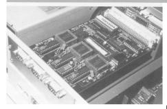
Based on the original design by The Serial Port, Atomwide's High Speed Serial Card enables users of most Acom Archimedes computers to take full advantage of modern, fast moderns. Furthermore, any Acom computer user with several serial devices can keep them all simultaneously connected, so removing the need to constantly swap cables or invest in a cumbersome manual switch box.
