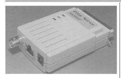
The Atomwide Network Printer Adaptor is a small device that connects between a 10base2 or 10baseT Ethernet point and the parallel port of any printer. On a network featuring a Windows NT server, printers attached to this small box can then be used by clients as if they were connected locally. As a result, the need for a dedicated printer server is eliminated, each printer can be located alongside any convenient network socket, and the server handles all print job queueing and spooling.
