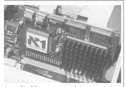
Acorn RiscPC users can turn their computers into powerful IBM compatible PCs with the addition of a 5x86 second processor card from Aleph One. Sharing memory, disk and display resources with the host computer, these PC cards give RISC OS users the ability to run most DOS and Windows software at speeds similar to those of a real PC.
