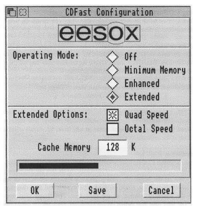
CDFast can be operated in one of three modes, "Minimum Memory mode", "Enhanced mode", "Extended mode" or CDFast may be turned off altogether. There are memory requirements and performance differences between the different modes, you should select the mode most appropriate. to your needs.
