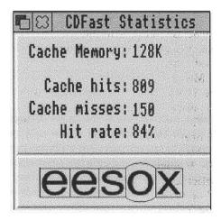
The statistics window shows you how well CDFast is working. It can be used to tailor the amount of cache memory to use. The higher the "Hit rate" the better. Anything over 30% is considered to be good, and will give speed good improvements.
