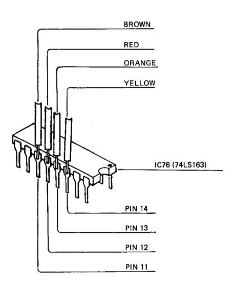
AFTER HAVING CONNECTED THE ROM BOARD PLEASE MAKE SURE THAT THE CONNECTIONS ARE TO THE DRAWING BELOW.
