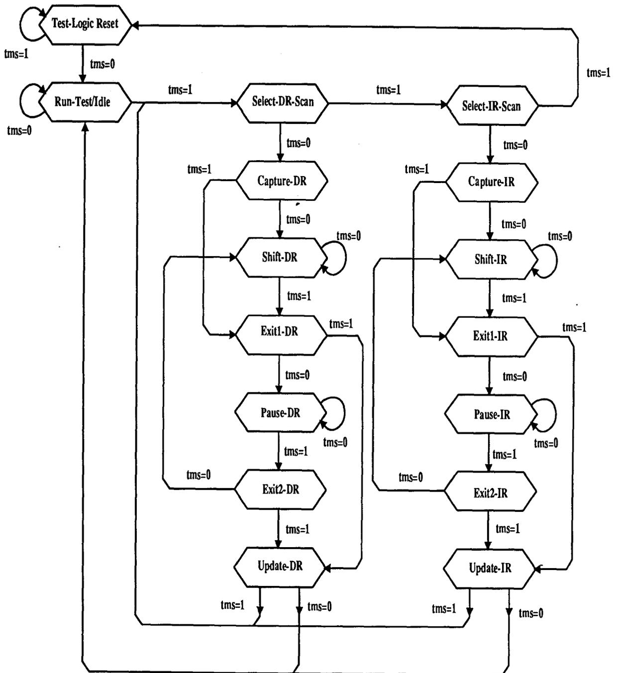
Figure 10.2 TAP Controller State Diagram
