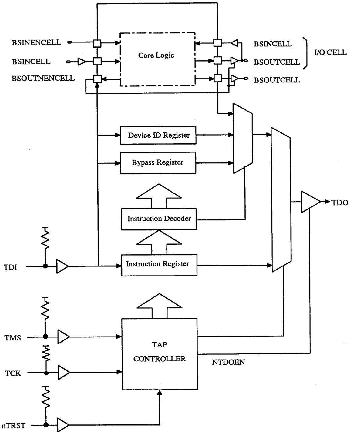
Figure 10.1 Boundary-Scan Block Diagram
