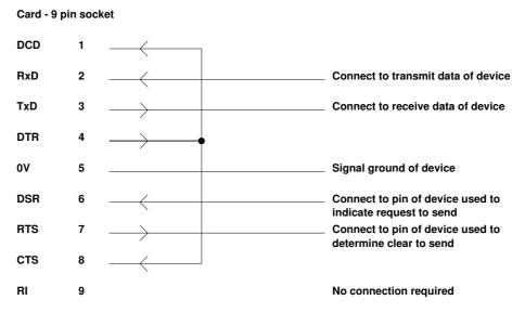
This cable wiring can also be used with the inbuilt port of any Acorn RISC OS-based computer.
