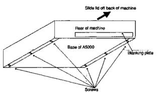
You should now remove the lid by sliding it firmly towards the rear of the machine.
