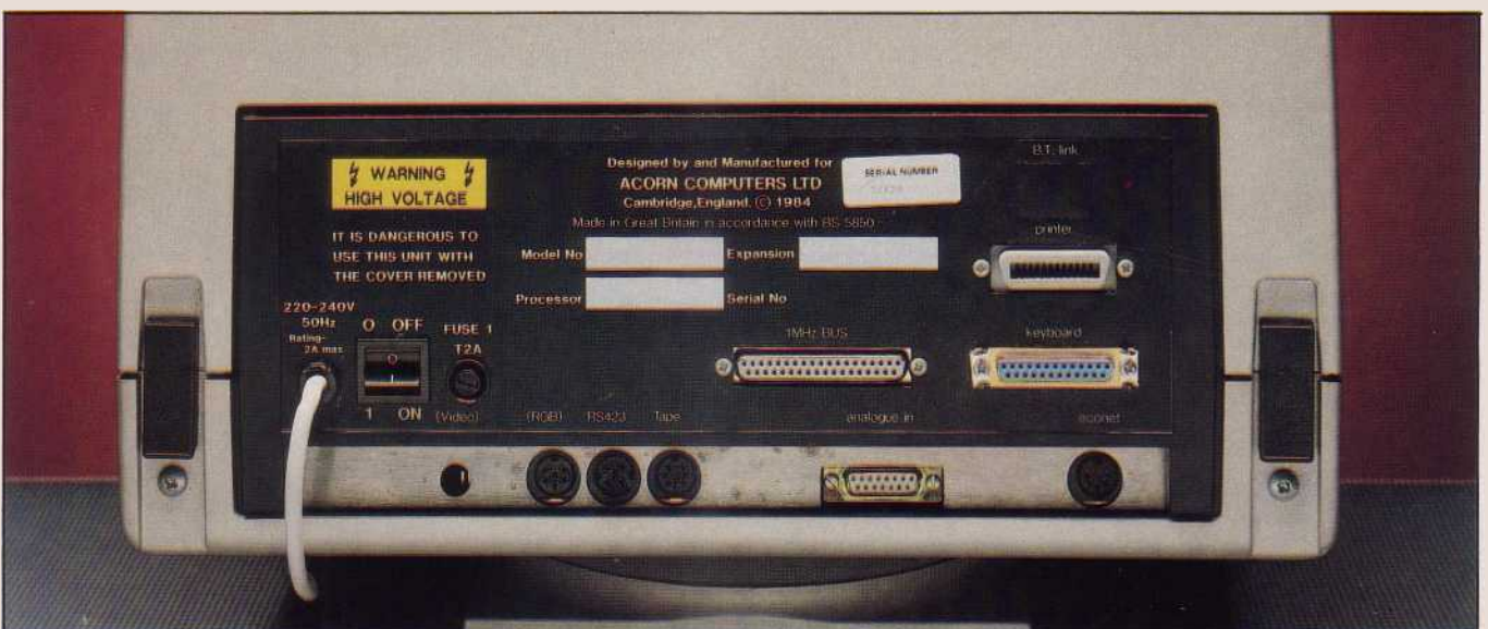
The back panel houses a wide range of I/O ports which are arranged on four levels in random order
