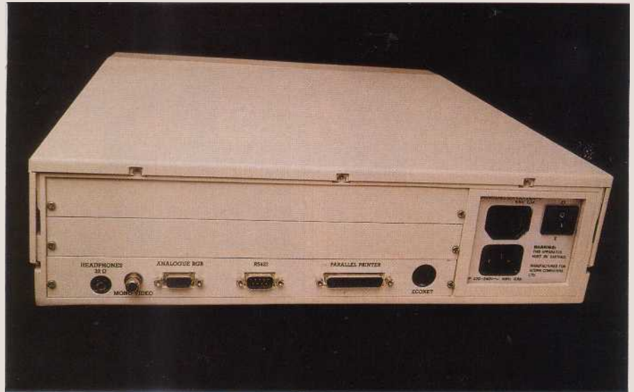
The back of the Archimedes is relatively sparse by today's standards, consisting of: headphone sockets, mono video out, analogue RGB, serial, parallel and Econet. The two removable plates above the ports will accommodate 'podules' —that is, peripheral modules
