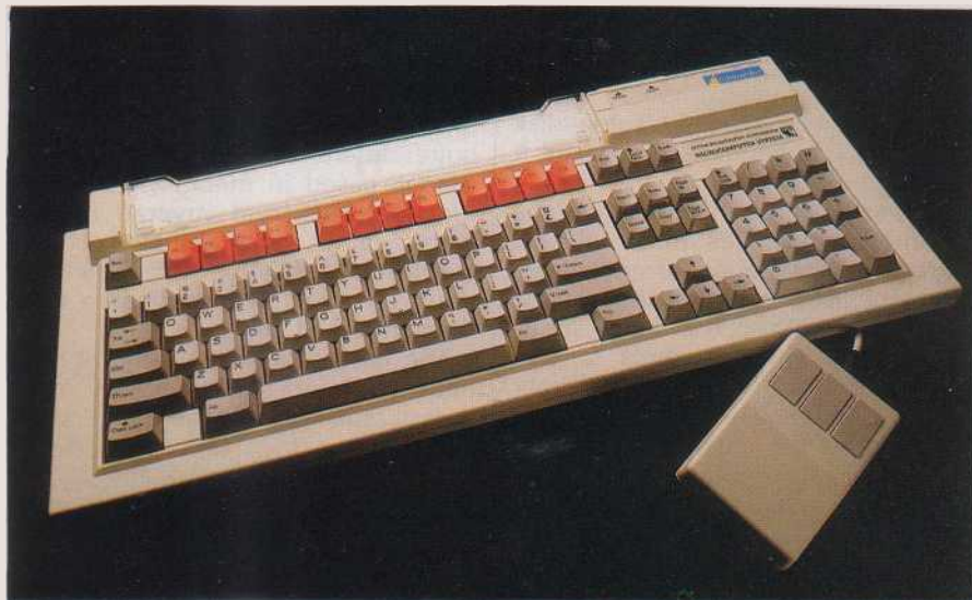
One concession to 'industry standards' is the Archimedes keyboard, which offers both IBM PC and BBC Model B compatibility. Like the Model 300 it has red function keys, presumably to persuade BBC Model B owners to 'upgrade' to an Archimedes. A threebutton mouse is fitted as standard
