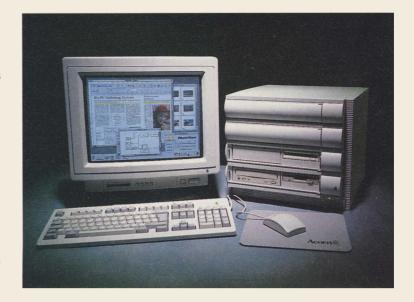
chip to access the screen memory. The RISC PC has solved most of these problems. Two 72-way SIMM sockets can be fitted with 128Mb DRAM in currently available packages, RISC OS 3.60 can address up to 256Mb and sound circuitry is cleaner. Up to 2Mb of on-board dual-ported VRAM is now addressable by a new ARM VidC20 chip, curing the ARM CPU wait state power drain.
