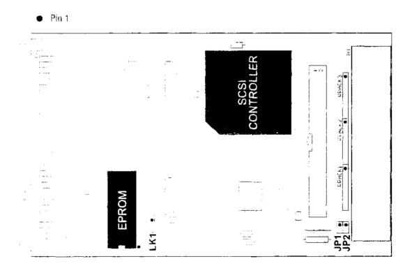
On the cached cards, three jumpers need to be set. LK1 set to 1-2, LK2 set to 2-3 and LK3 set to 1-2, and insert EPROM.
