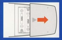
**2** Install three AAA batteries into the compartment, ensuring that you observe the correct polarity positions.
