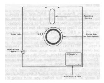
The disc will be in a paper or cardboard protective envelope. Whenever a disc is not being used, return it to its envelope, and then to a suitable storage box, to protect it from dust. Dust can not only destroy a floppy disc and the information on it, but it can wreck the disc drive as well.
