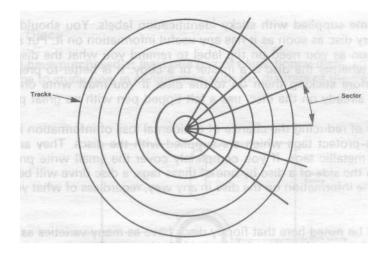
Each sector contains 256 data bytes, plus some control information. Thus a 40-track disc recorded in single density will hold 40\*10\*256 = 100K bytes of data per side, similarly an 80 track disc recorded in double density will hold 80\*18\*256 = 360K bytes of data per side.
