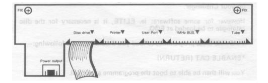
If there is a 6-way power connector, this should be connected to the socket marked 'Auxiliary power socket'. It is not possible to connect this plug in other than the correct orientation. If the drive unit has its own power supply, plug in the mains power lead.
