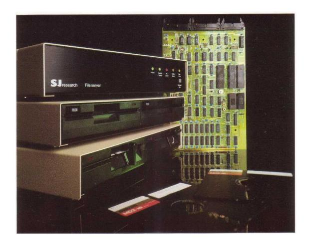
The FDFS is a purpose designed floppy-disc file server. One neat and unobtrusive box offers all the services required for a small or medium sized network, providing both a file server and two printer servers.
