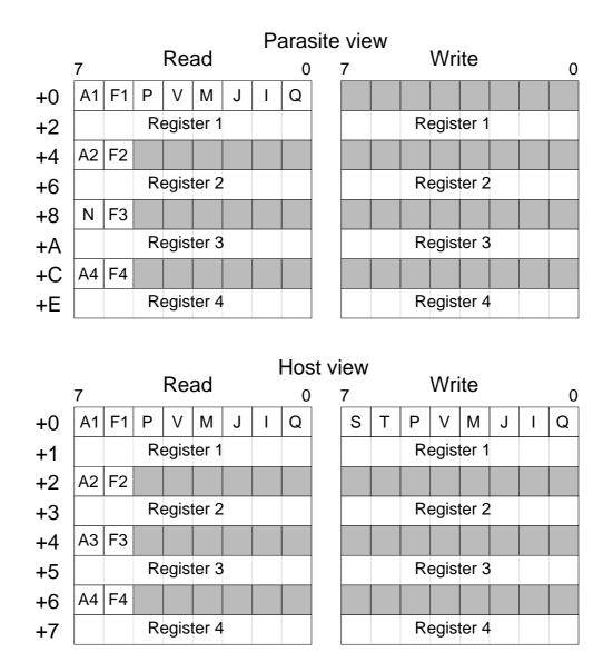
Note that for the parasite register layout, the byte wide registers are spaced on 16 bit boundaries in hardware, so must be accessed using LDRB (or LDRH) to avoid accessing two registers at once.
