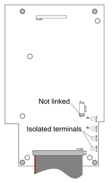
Locate the pair of power terminals and connect the +5V supply lead (usually red) to PL103 and 0V or ground (usually black) to PL104. Two spare terminals, not normally fitted, are available to secure any unused power cables from the integral power supply - these are isolated.
