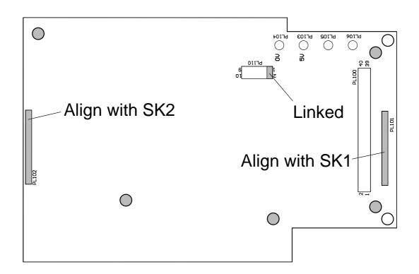
Five holes (shaded above) can be used to lock the coprocessor in place using 18mm PCB standoffs (not supplied) if required, otherwise replace the lid and fixing screws.
