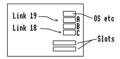
Use socket B if possible, or alter Link 19 to East to use A, or alter Link 18 to East to use C: this will however result in a loss of some sideways RAM.
