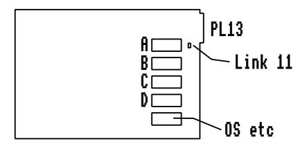
first move Link 11 to South, note any upgrades on PL13 will be disabled as a result of this so try to use A, B, C first.
