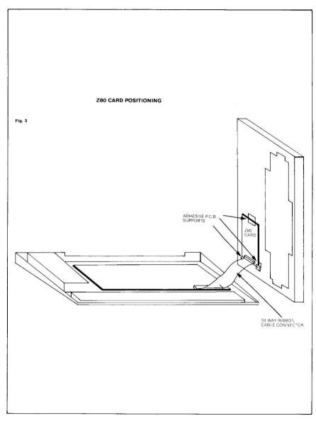
the box. It is important to mount the Z80 card in this manner so that the 200mm cable provided will be of sufficient length to connect the Z80 card to the TUBE interface on the BBC machine. The following procedure should then be followed.
