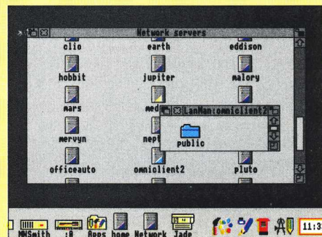
Via OmniClient all protocol modules loaded make another range of file servers available
