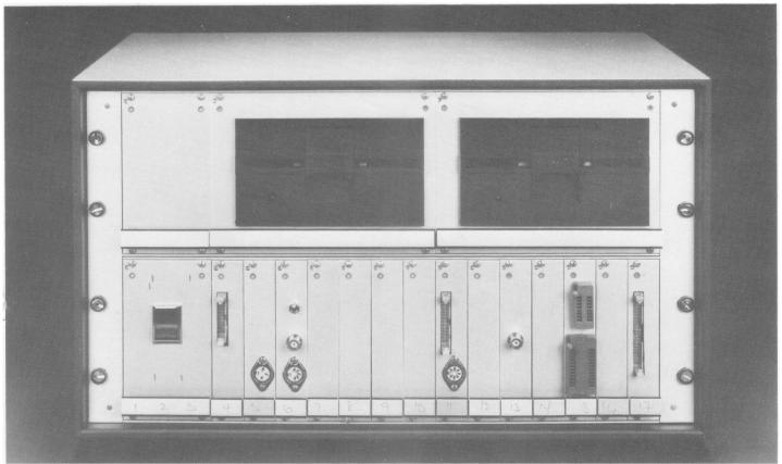
The Acorn System 4 Computer is housed in a double height rack with facilities for up to 14 Eurocards. The basic system has as standard two floppy disk drives, power supplies, card frame buffered backplane, 6502 CPU, VDU interface, 16K RAM and disk controller. A Disk Operating System controls both disk drives and a disk with utilities programs including disk copy is supplied with each system.
