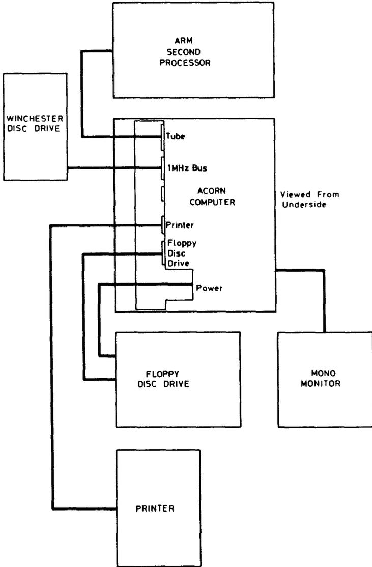
The cable supplied with the co-processor is captive at the co-processor end and has a 40-way IDC connector at the other end which plugs into the interface, under the BBC Model B or BBC Master microcomputer, marked TUBE. The co-processor has a separate mains lead for connection to a 240 V 50 Hz mains supply.
