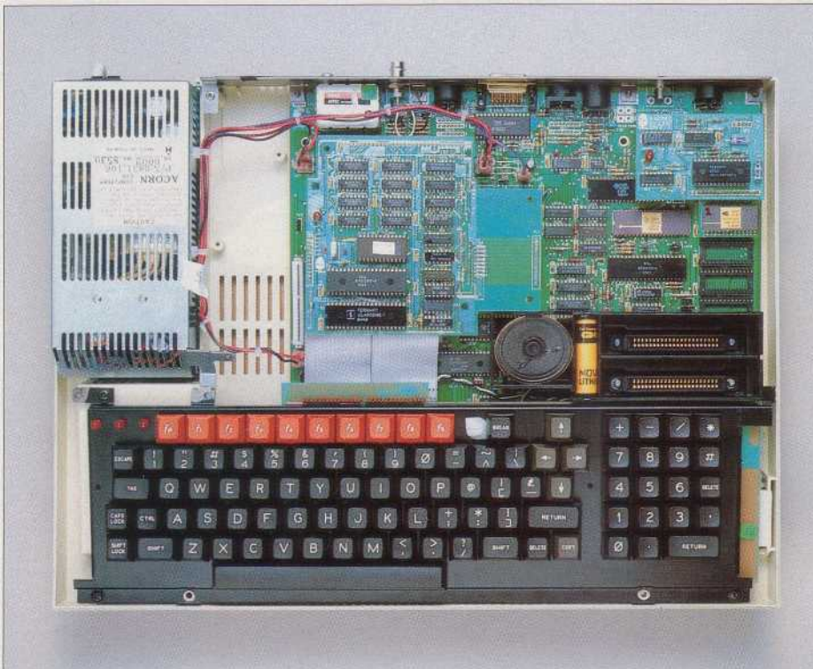
Inside the Master 128: this model has the Turbo co-processor and Econet interface fitted
