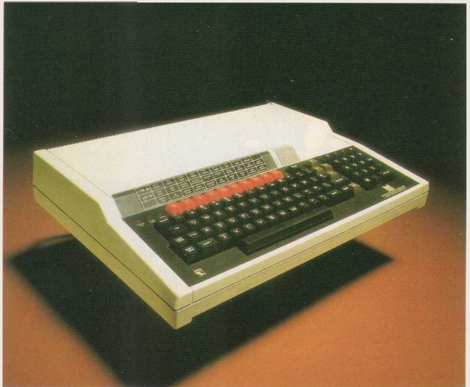
The Master 128: the cornerstone of Acorn's new range of micros which can be upgraded with co-processors
