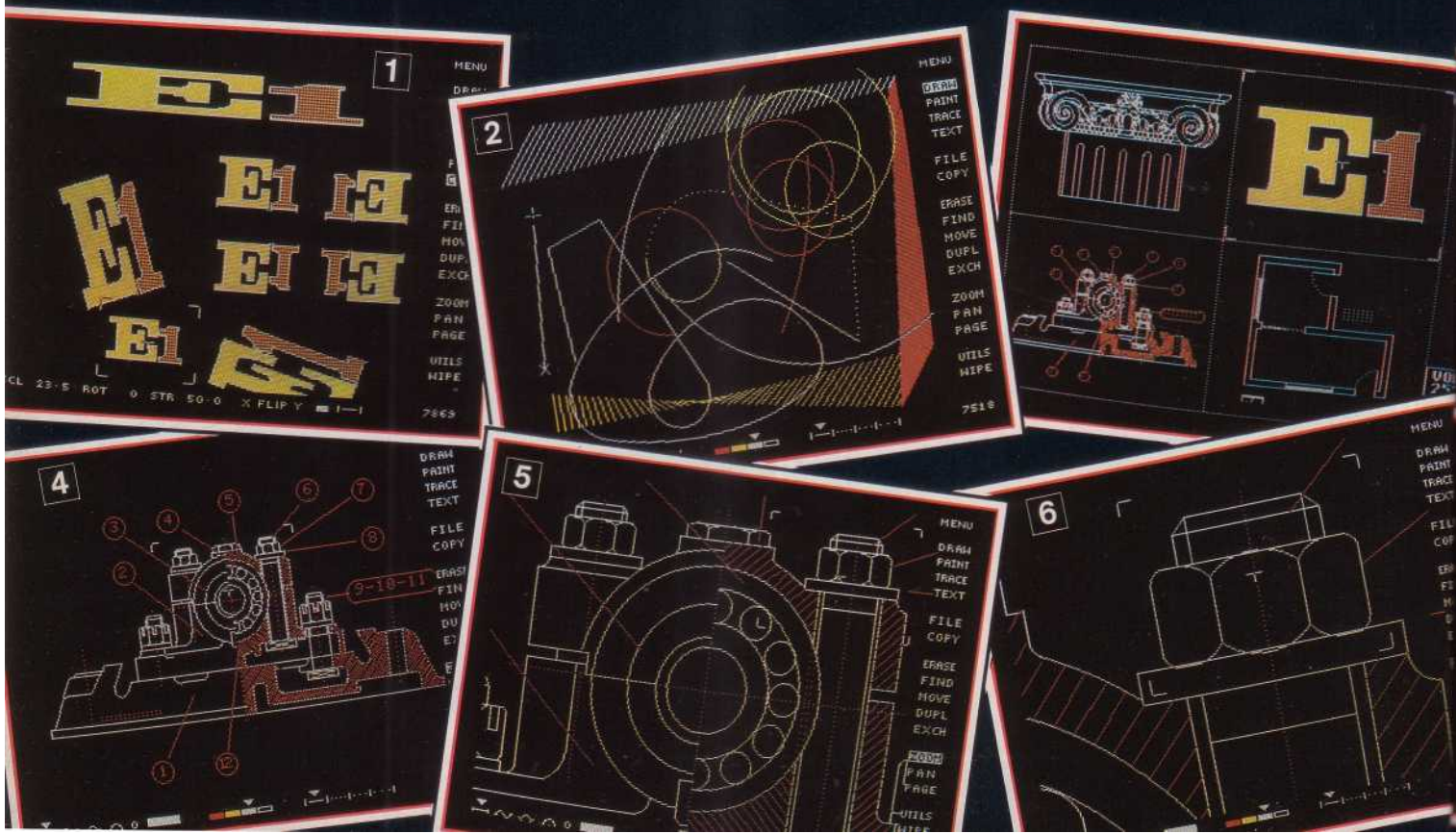
Screen shots from Bitstik system. 1. Manipulation and distortion of any image is possible, in this case of the lettering in picture 9. Menu at bottom gives information on distortion. 2. Arty doodles at your fingertips. Base menu shows colour and drawing mode chosen. 3. Disc menu. Top right image has been chosen for copying. Note change in menu. 4, 5, 6. Zoom, zoom, zoom. Level of detail in image held is virtually unlimited.
