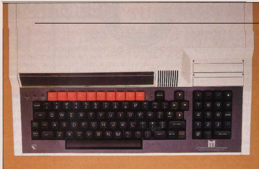
The keyboard features a cursor key diamond—a big improvement over the BBC B
