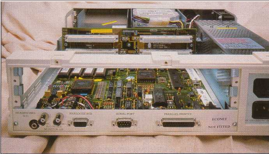
Under the lid the hardware is virtually identical to the Archimedes 440, with the only additions being the new disk drive, the four RISC OS ROMs and the expansion ( module) card
