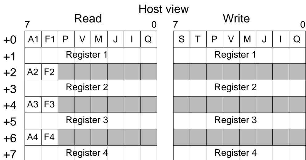
Note that for the parasite register layout, the byte wide registers are spaced on 16 bit boundaries in hardware, so must be accessed using LDRB (or LDRH) to avoid accessing two registers at once.
