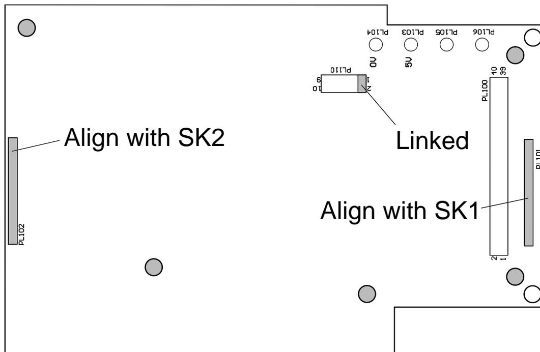
Five holes (shaded above) can be used to lock the coprocessor in place using 18mm PCB standoffs (not supplied) if required, otherwise replace the lid and fixing screws.
