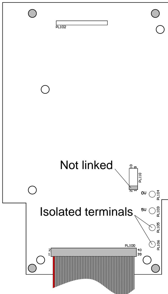
Locate the pair of power terminals and connect the +5V supply lead (usually red) to PL103 and 0V or ground (usually black)
