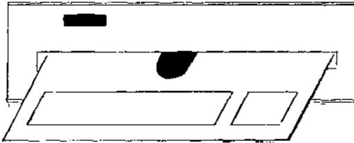
When the disc is flush with the front of the drive, push the button just above the slot in until it clicks. Note that the button stays in almost flush with the fascia.
